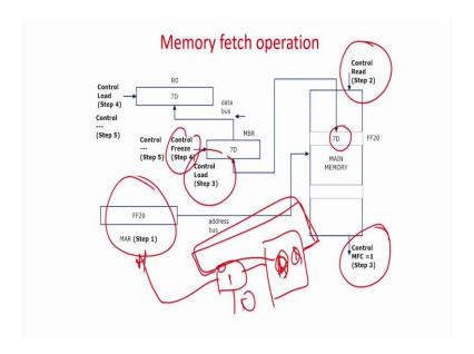
So, now let us see step one. So, I want to read from this memory location FF20. So, memory address register will have the value of FF20, this is connected to the address bus it is going then I want to read this basically. So, now, next step is read, read signal is given now you have to wait how you have to wait till memory function complete is one. So, once the memory functions complete is 1, it means that the value of this one is written to the memory buffer register and it is stable.
